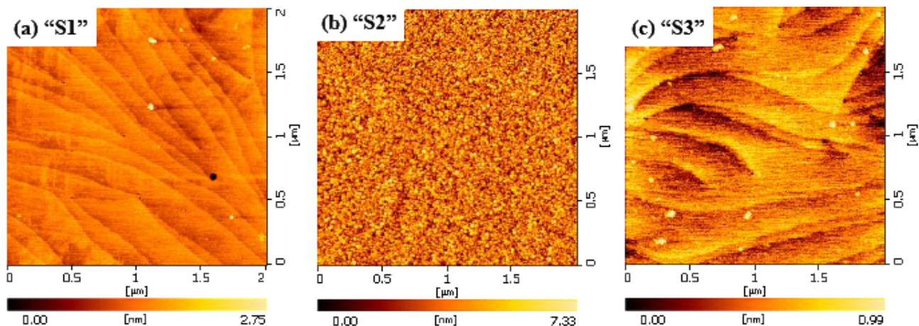
**Figure 3.** The surface morphology of samples (a) ‘S1’: untreated GaN films; (b) ‘S2’: after 100 s TMGa flow over the surface of ‘S1’ in  $H_2$  and  $NH_3$  ambient at  $500^\circ C$  and 500 Torr; (c) ‘S3’: 800 s TMGa flow over the surface of ‘S2’ in  $H_2$  and low  $NH_3$  ambient at  $1035^\circ C$  and 300 Torr (GaN droplet homoepitaxy).
