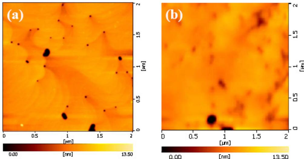
Figure 8. The surface morphology of samples (a) 'WB1': with GaN cap layers on 'W1'; (b) 'WB3': with GaN cap layers on 'W3'.
