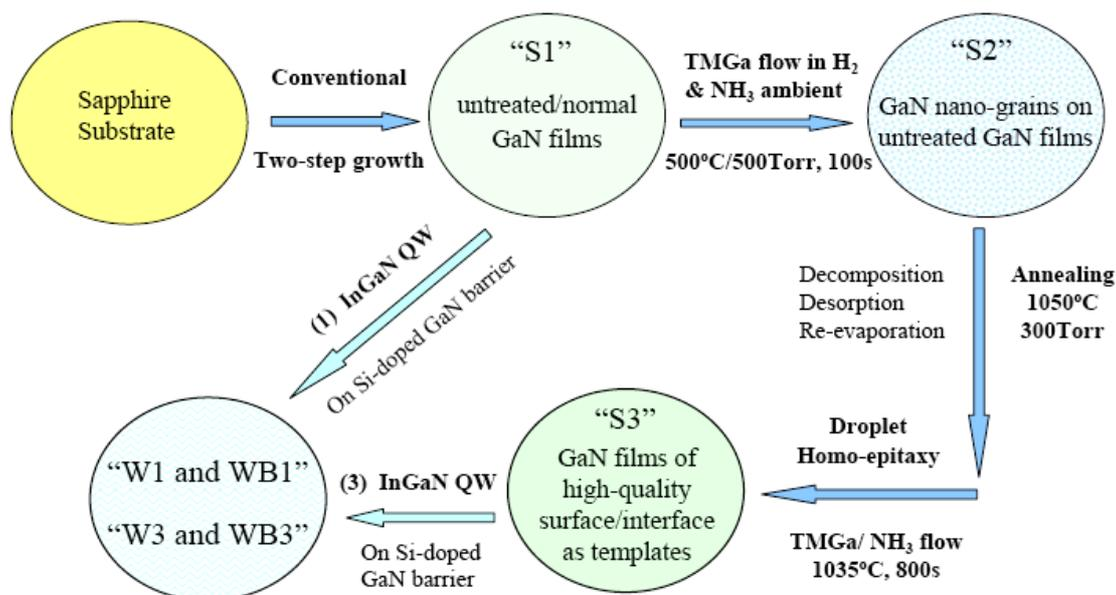
**Figure 2.** Schematic diagram for the preparation procedures of the InGaN/GaN SQW on treated and untreated GaN films. In the figure, 'S1', 'S2' and 'S3' stand for GaN films at different treatment and growth stages, 'W1' and 'W3' for InGaN epilayers on the untreated and treated GaN films, and 'WB1' and 'WB3' with GaN cap layers on 'W1' and 'W3', respectively.
