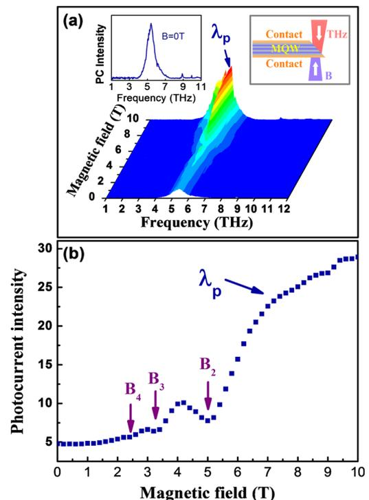
FIG. 1. (Color online) (a) PC spectrum for the GaAs/Al<sub>0.03</sub>Ga<sub>0.97</sub>As QWP under magnetic field from 0 to 10 T at liquid helium temperature. The left inset shows the zero-magnetic-field PC spectrum. The right inset shows the measurement geometry. (b) Magnetic field dependence of PC intensity at peak response  $\lambda_p$ . Intensity resonance of  $\lambda_p$  are marked with arrow B<sub>2</sub>, B<sub>3</sub>, and B<sub>4</sub>.
