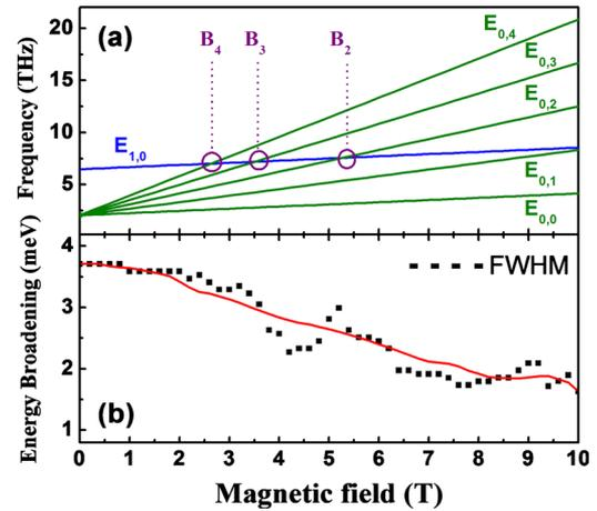
FIG. 3. (Color online) (a) Landau levels in magnetic fields for the GaAs/Al<sub>0.03</sub>Ga<sub>0.97</sub>As QWP. Intensity resonances at magnetic field of  $B_2$ ,  $B_3$ , and  $B_4$  satisfy condition of  $\varepsilon_{1,k} - \varepsilon_{0,l} = n\hbar\omega_c$  ( $n=2, 3$ , and  $4$ ). (b) Magnetic field dependence on linewidth (FWHM) of PC spectrum for the GaAs/Al<sub>0.03</sub>Ga<sub>0.97</sub>As QWP. Short-dashed line is used for visual aid only.
