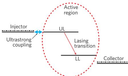
**Figure 1** | Key physical process in the Gmachl study<sup>2</sup>. The active region includes an upper lasing state (UL) and a lower lasing state (LL). The injector state couples with the upper lasing state by tunnelling. The ultrastrong coupling regime corresponds to a narrow tunnel barrier.
