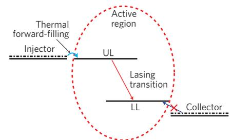
**Figure 2** | Key physical process in the Razeghi study<sup>3</sup>. When the separation between the lower lasing state and the collector region chemical potential is small, thermal back-filling is negligible at low temperatures. Moreover, at such temperatures, thermal forward-filling is possible from the injector state to the upper lasing state. Both mechanisms favour a lower voltage defect and therefore a higher wall-plug efficiency.
