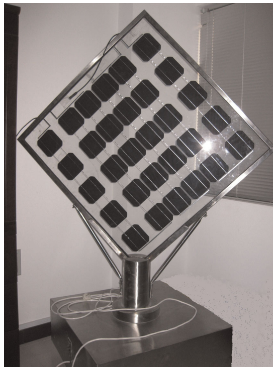
Figure 6. Appearance of the glass–glass, 30 bifacial cells PV module fabricated for this study.
