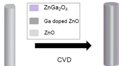
Fig. 8 A proposed three-layer nanowire structure of ZnO core, Ga-doped ZnO middle-layer, and ZnGa 2 O 4 shell
