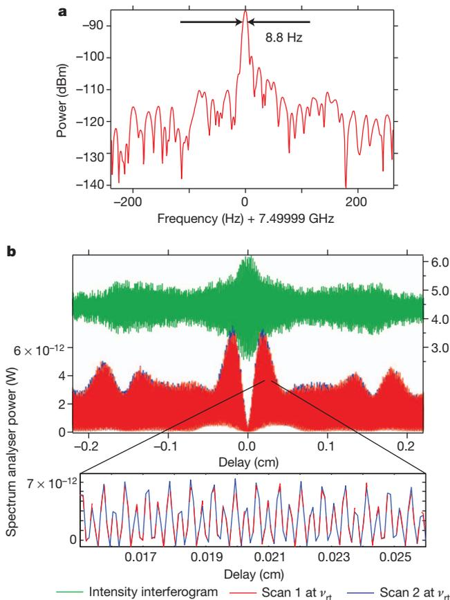
**Figure 2 | Intermode beat spectroscopy.** **a**, Narrow intermode beat, with a full-width at half-maximum of  $<10\text{ Hz}$  at the onset of the multimode emission. The resolution bandwidth of the spectrum analyser is set to 10 Hz. **b**, Intensity interferogram and intermode beat interferograms measured in two successive scans separated by 90 min, at 490 mA. The resolution bandwidth is 100 kHz. QWIP, Quantum-well infrared photodetector. **c**, Comparison of the measured
