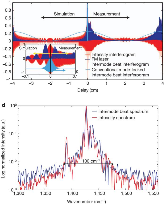
intermode beat interferogram at 480 mA with two intermode beat interferogram simulations of a perfectly frequency-modulated (FM) signal and a fundamentally mode-locked laser. Inset, magnified view of region at zero delay. **d**, Comparison of the intermode beat spectrum,  $\mathcal{J}(\nu_{\text{rt}}, \omega)$ , and the intensity spectrum,  $\mathcal{J}(0, \omega)$ , at an injection current of 500 mA.
