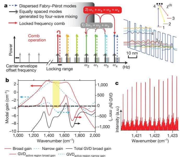
**Figure 1 | Optical frequency comb in a quantum cascade laser.** **a**, The dispersed Fabry–Pérot resonator modes lock to the equally spaced modes generated by four-wave mixing processes. **b**, Gain and GVD simulations of a narrowband (dotted) and a broadband (solid lines) quantum cascade laser. **c**, Magnified view of the laser spectra at  $I = 740$  mA, measured using a high-resolution Fourier transform infrared spectrometer ( $0.0026 \text{ cm}^{-1}$ , 78 MHz). a.u., arbitrary units.
