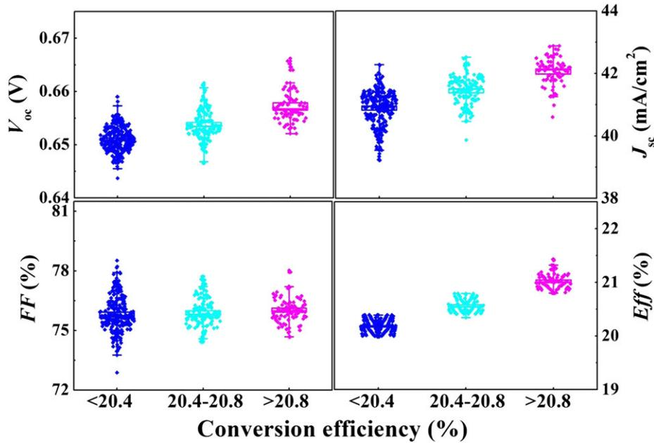
**Figure 7.** Electrical parameters ( $V_{oc}$ ,  $J_{sc}$ ,  $FF$  and  $Eff$ ) statistical distribution for the 445 pieces of the BJBC silicon solar cells with size of  $6 \times 6 \text{ cm}^2$  under the three different grades of the conversion efficiency. [Colour figure can be viewed at [wileyonlinelibrary.com](http://wileyonlinelibrary.com)]
