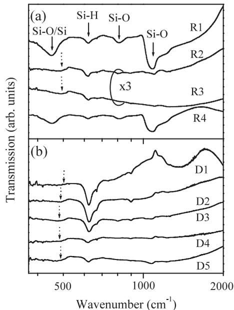
**Figure 3.** Room-temperature IR transmission spectra for the two sets of nc-Si:H thin film samples. The spectra of samples R2 and R3 have been multiplied by a factor of three for clarity.
