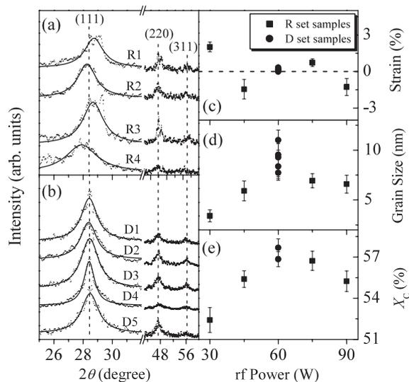
**Figure 2.** X-ray diffraction patterns for the (a) R set and (b) D set nc-Si:H thin films. The resultant average (c) lattice strain, (d) grain size from the Lorentz fitting of the (111) diffraction peak, and (e) crystalline fraction  $X_C$  from the Raman measurements.
